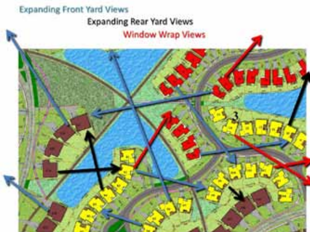
The angle relationship between homes of a coved design increases length of views from within the homes.
